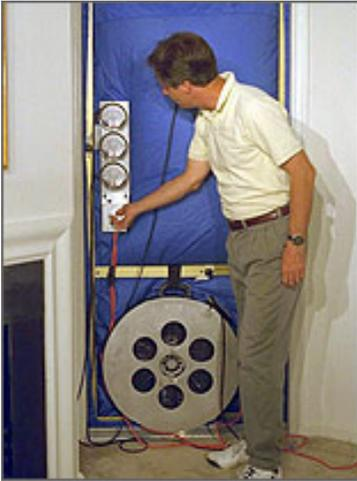
Blower door tests are often used in energy audits to determine the airtightness of a residence.
