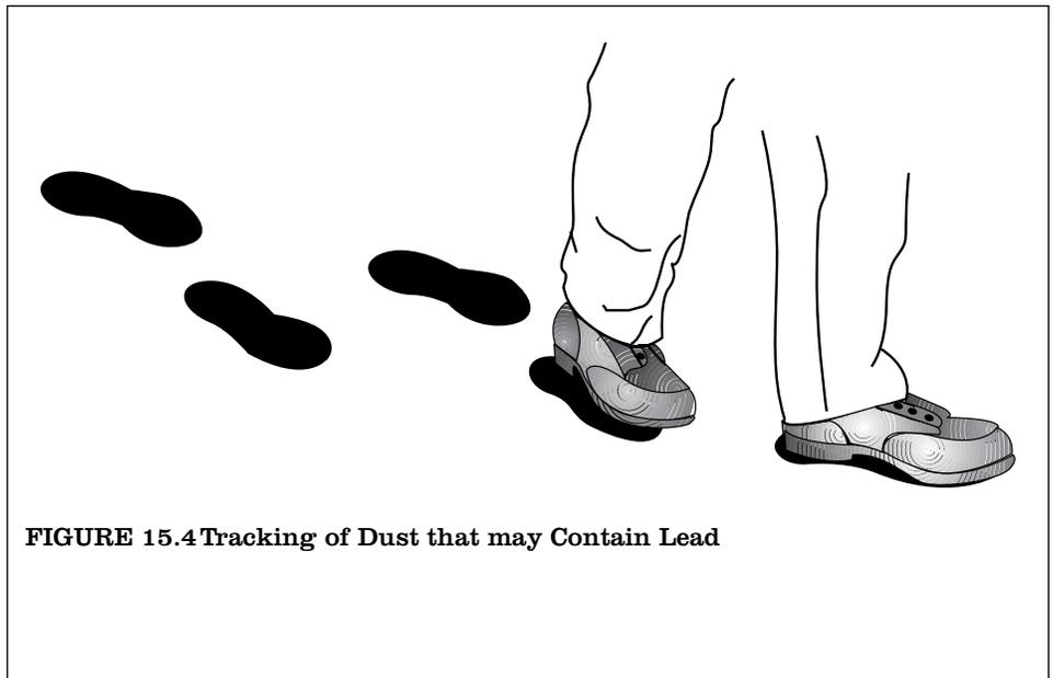
**FIGURE 15.4** Tracking of Dust that may Contain Lead
